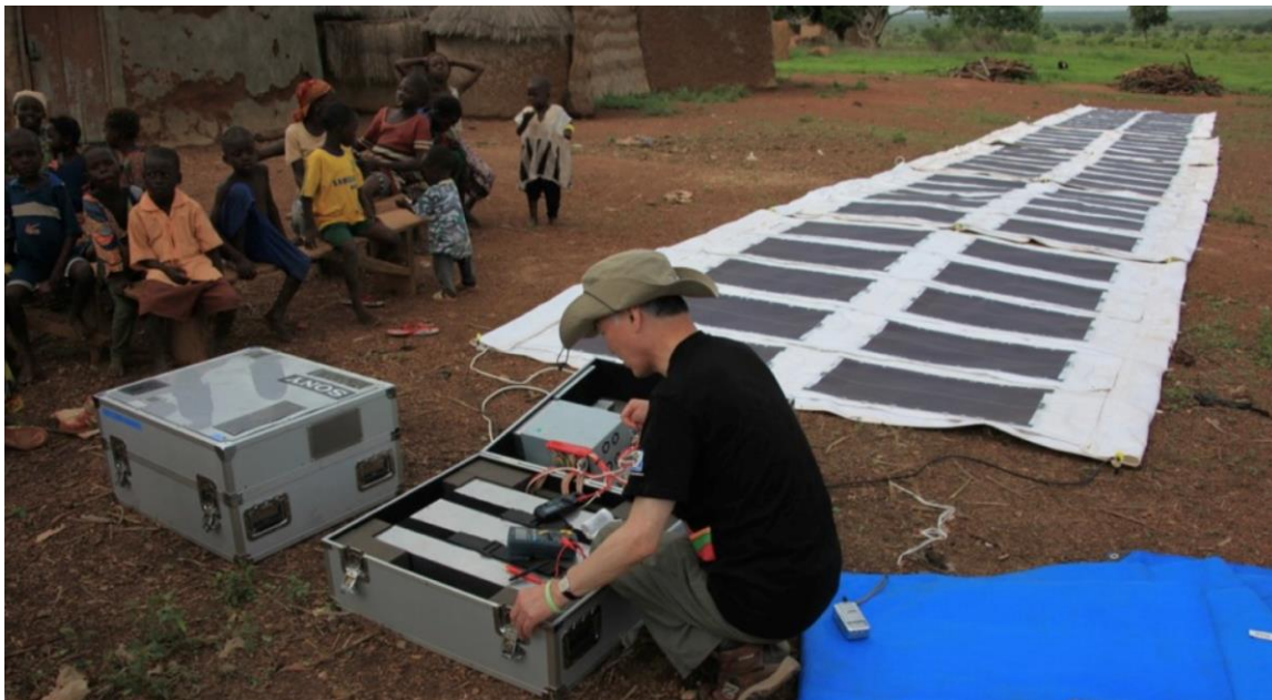
Figure 1. Technologies required to collect blood samples: solar panels to generate electricity in rural areas with no electricity, and batteries to store electricity for night-time use and provide refrigeration for the blood samples.
