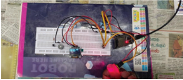
Fig. 3. Output design of the patient monitoring system shows how the health data, such as SpO 2 and HR, are monitored during the system testing phase, enabling the evaluation of output accuracy and system performance. HR: heart rate; SpO 2 : peripheral oxygen saturation.
